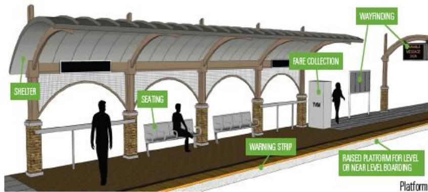
Comfortable transit stations with weather protection, seating, lights, and ticket vending machines
